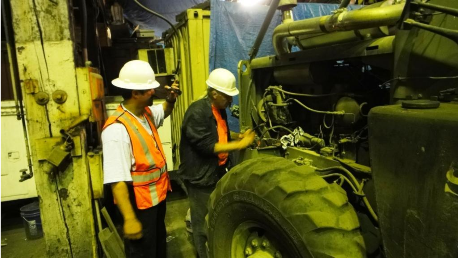
Jose and Fred take the batter cables apart on the Green Machine
